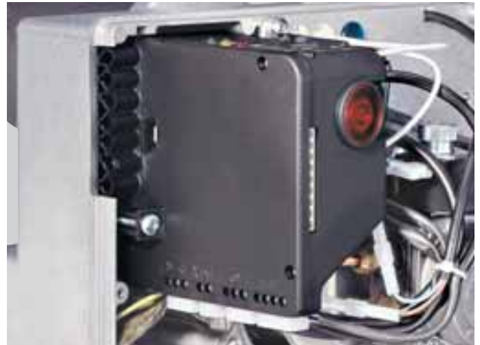
Control box fitted with ignition transformer
